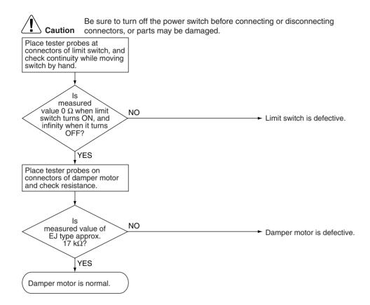
Check resistance and voltage - DAMPER MOTOR
