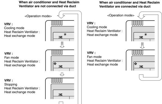
Note) Current Ventilation mode can be visible and selected on the remote controller.
