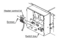
Take off the screws on the terminal plate. Turn up the terminal plate as shown below.
