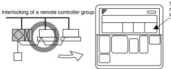
The display and operation of a remote controller is the same as a standard indoor unit.
