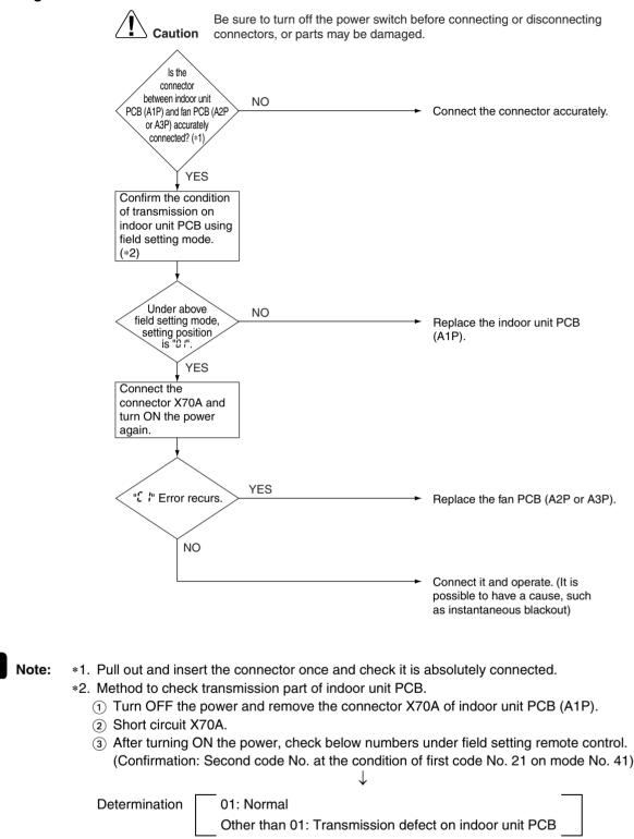
\* After confirmation, turn OFF the power, take off the short circuit and connect X70A back to original condition.
