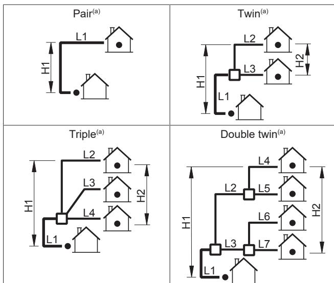
(a) Assume that the longest line in the illustration corresponds with the actual longest pipe, and the highest unit in the illustration corresponds with the actual highest unit.
