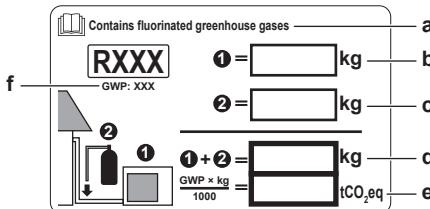
a If a multilingual fluorinated greenhouse gases label is delivered with the unit (see accessories), peel off the applicable language and stick it on top of a.
