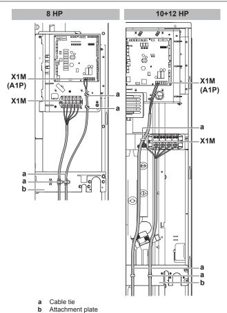
Power supply Transmission wiring X1M (A1P)
