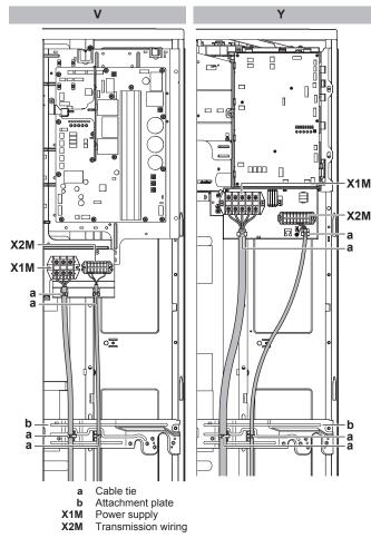
Route the wiring through the frame and connect it to it.
