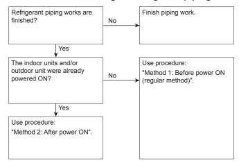
It is very important that all refrigerant piping work is done before the units (outdoor or indoor) are powered on.
