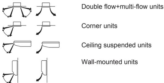
For the following conditions, a micro computer controls the air flow direction which may be different from the display.
