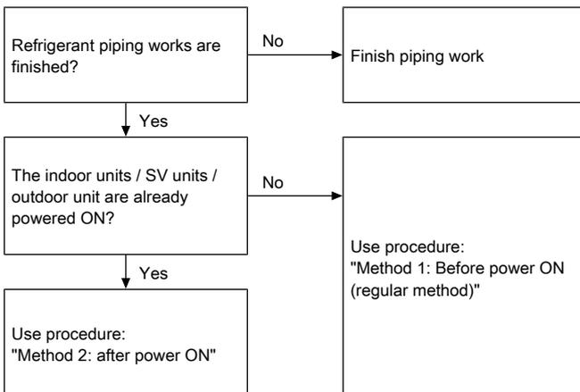
It is very important that all refrigerant piping work is done before the units (outdoor, SV unit or indoor) are powered on. When the units are powered on, the expansion valves will initialise. This means that the valves will close.
