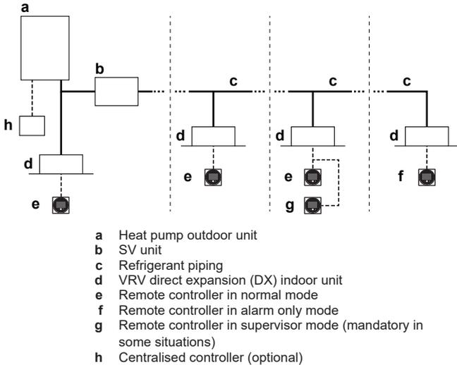
**Note:** During start-up of the system, the mode of the remote control can be verified from the screen.
