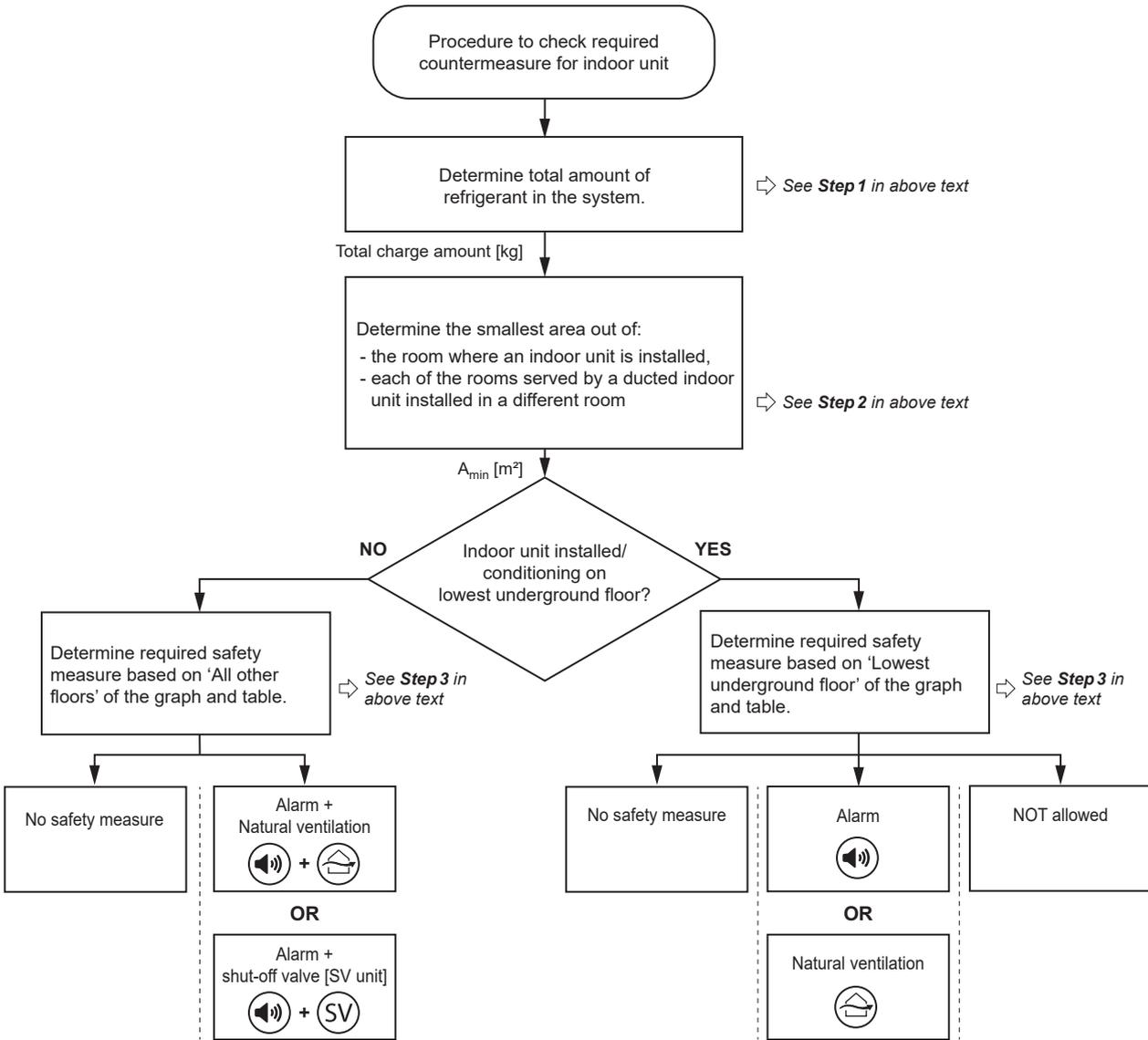
**Note:** The flowchart is an overview. Always refer to the full text mentioned in this manual for clear understanding and detailed explanation.
