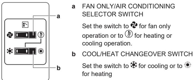
**Note:** In case a cool/heat changeover remote control switch is used, the position of DIP switch 1 (DS1-1) on the main PCB needs to be switched to the ON position.
