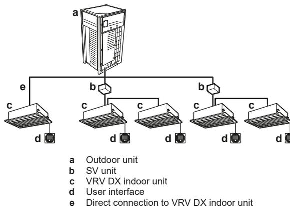
When the system is installed as shown in the figure above, it is necessary to – for each subsystem – designate one of the user interfaces as the master user interface.
