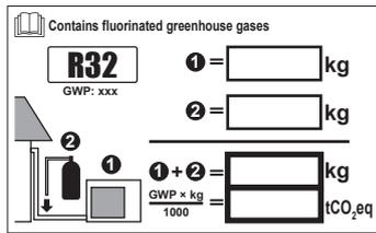
Total charge=Factory charge ①<sup>(a)</sup>+additional charge ②<sup>(b)</sup>
