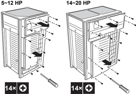
Once the front plates open, the switch box can be accessed. See "14.2.2 To open the switch box of the outdoor unit" [p. 28].
