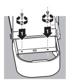
If the unit is in danger of falling over, either fasten to the wall using the holes provided, or fasten to the floor with a field supplied floor fastener.
