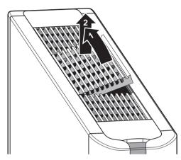
Lift the rear using the front as a leverage. To install use the opposite method.
