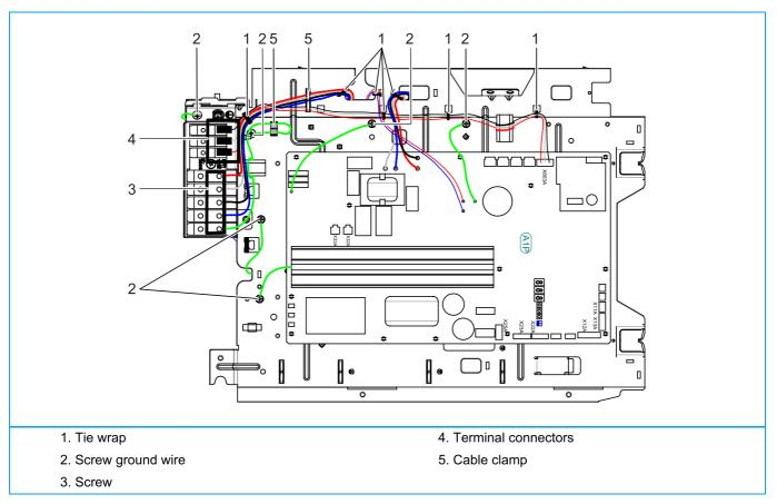
Finally, strip the Main PCB assembly (rear)
