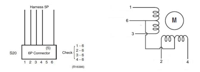
3. If one or more of the windings have no continuity, replace the expansion valve coil.
