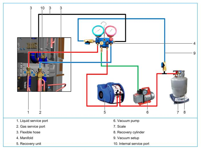
5. Activate vacuum mode via the field settings (see field settings in installation manual or installer reference guide).
