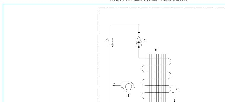
Figure 5-15: Piping diagram - indoor unit FBA
