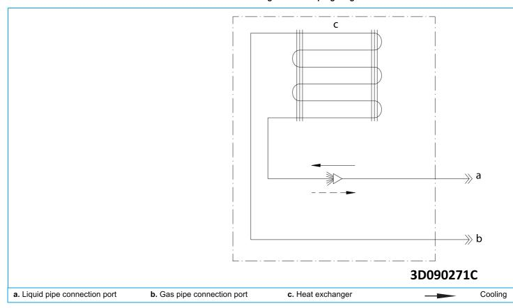
Figure 5-16: Piping diagram - indoor unit FDA
