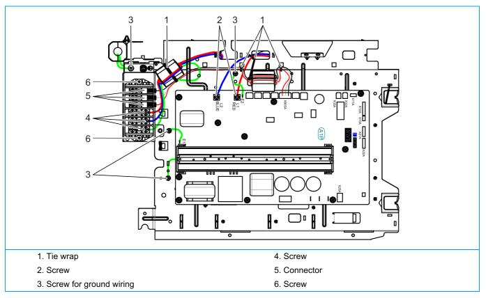
Finally, strip the Main PCB assembly (rear)
