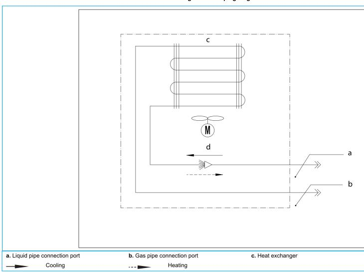
Figure 5-17: Piping diagram - indoor unit FFA
