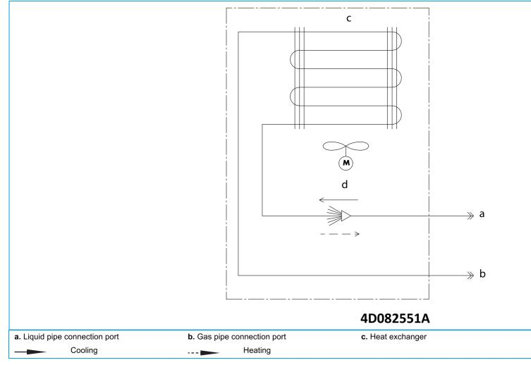
Figure 5-18: Piping diagram - indoor unit FHA
