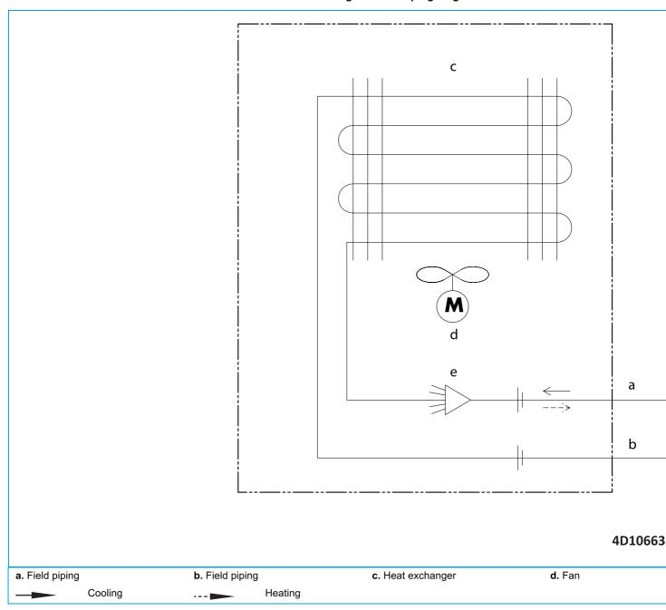
Figure 5-21: Piping diagram - indoor unit FVA
