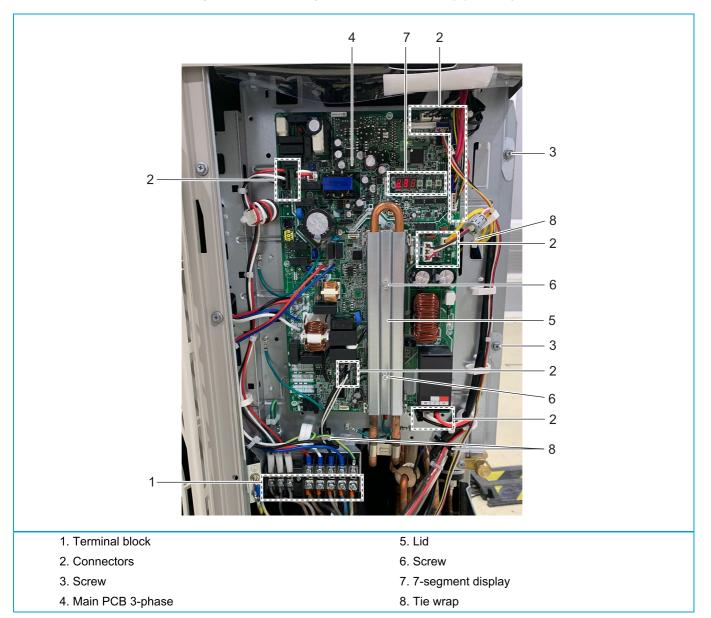
Secondly, strip the Main PCB assembly (front)
