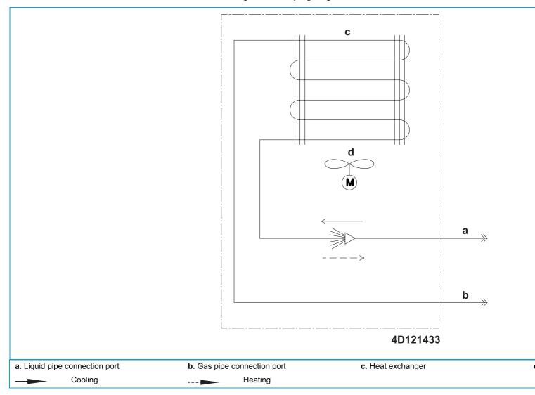
Figure 5-14: Piping diagram - indoor unit FAA
