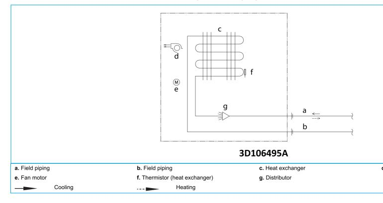
Figure 5-19: Piping diagram - indoor unit FNA
