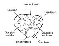
2. Be sure to insulate both the gas and liquid piping and to provide insulation dimensions as below.
