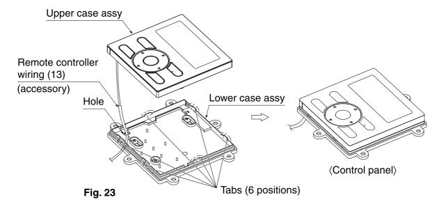
2. Remove the front panel, and then remove the back plate attached to the back side.
