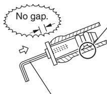
Do not apply lubricating oil (refrigerant oil) to the drain plug when inserting it. The application of lubrication oil to the drain plug will deteriorate the plug to cause drain leakage from the plug.
