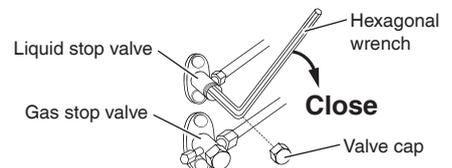
After the operation, reattach the valve cap to the original condition.
