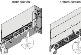
3 Clean the air filter. Use a vacuum cleaner or wash with water.
