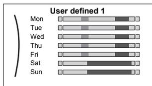
**Prerequisite:** The room temperature schedule is only available if room thermostat control is active. If leaving water temperature control is active, you can program the main zone schedule instead.
