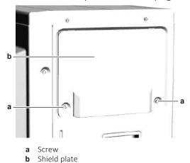
**12** Install the shield plate and secure it by tightening the two screws.
