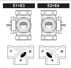
**3** When installing in accordance with configurations E3 or E4, open the valve motor cover by loosening the screw and change the jumper so as to change the rotation direction of the valve.
