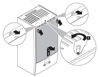
If you have to connect electrical wiring, remove the switch box cover.
