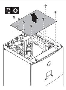
Remove the user interface panel. Open the hinges at the top and slide the top panel upwards.
