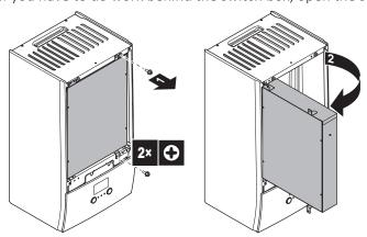
If you have to do work behind the user interface panel or upload new software into the user interface, open the user interface panel.
