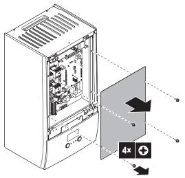
If you have to do work behind the switch box, open the switch box.
