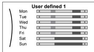
**Prerequisite:** The room temperature schedule is only available if room thermostat control is active. If leaving water temperature control is active, you can program the main zone schedule instead.
