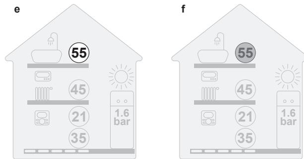
e Tank heating operation ON
