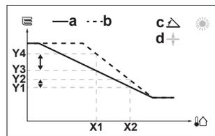
**Offset.** When offset is changed, the new preferred temperature at X1 is equally higher as the preferred temperature at X2.
