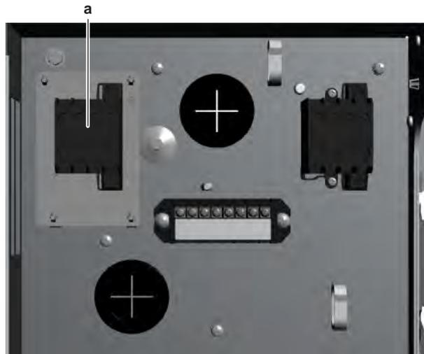
a Booster heater contactor K3M
