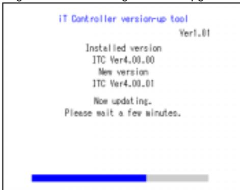
Figure 7 Screen during Software Upgrade
