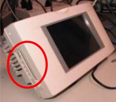
Figure 2 Reset Switch Position
