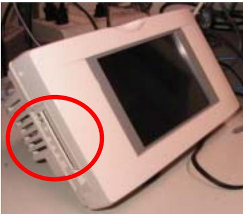
Set a switch to enable the use of a data backup battery. When this switch is already set, the screen shown in Figure 1 does not appear. In this case, proceed to the setup operations on the next page.
