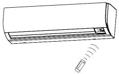
2 short beeps from the receiver indicates that the transmission is properly done. Transmitting distance is approximately 7 m.
