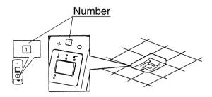
Operate the indoor unit with the remote controller of the same number.
