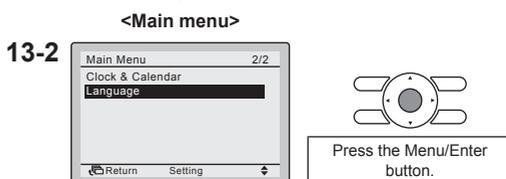
**13-3** Press the ▲▼ (Up/Down) buttons to select the desired language and press the Menu/Enter button. The settings are confirmed and the Basic screen returns.
