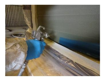
Copper elbows (returns), headers and brazing parts can be pre-treated with a special Polyurethane primer to ensure maximal adhesion and protection to these areas.
