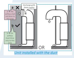
For non-ducted units in a "radiator style" box, a clear air path between the vertical and 55° is required and 100% of the return and supply airflows must go to/from the same room without using the enclosure as a plenum.
