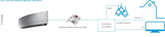
Connect Sky Air / VRV indoor units to KNX interface for BMS integration
